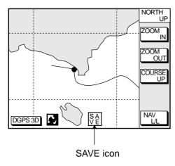
Figure 7-9 SAVE icon appearance on the plotter display
